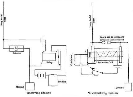
FIG. 175. Elements of a simple Wireless Telegraph Circuit.
